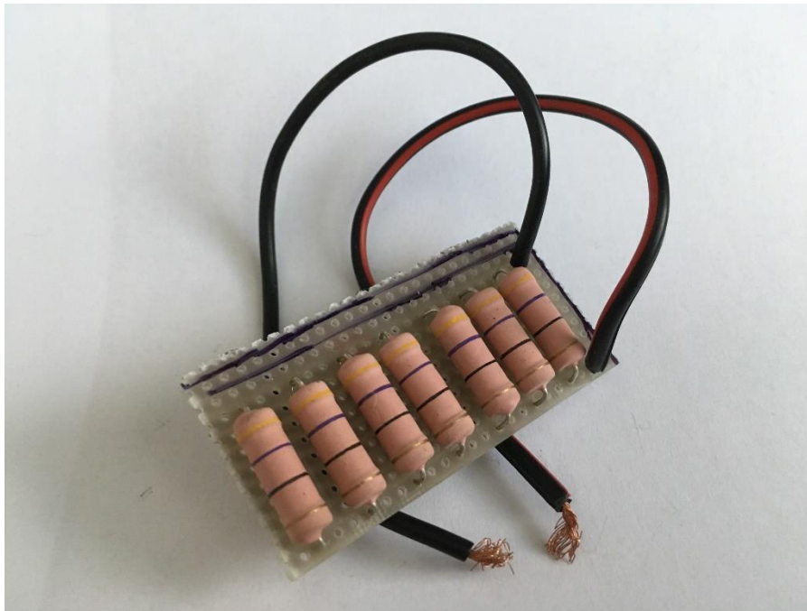
Picture 17 - First model of heater for testing heating in chamber
