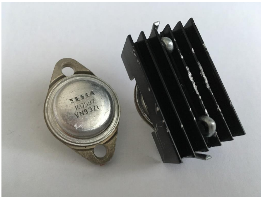
Picture 10 - Power transistor with mounted heatsink
