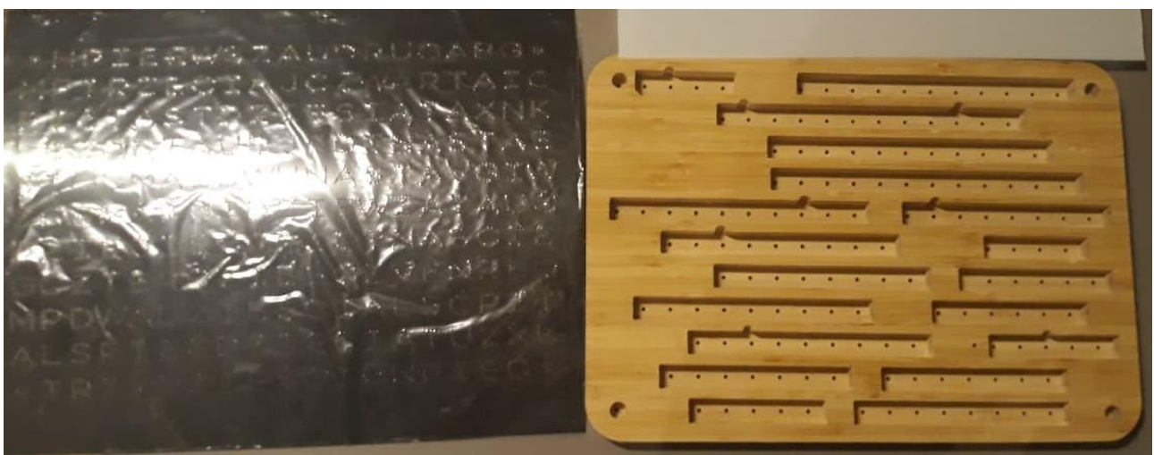
Polish board with milled holes for LEDs and black plastic plate with milled words
