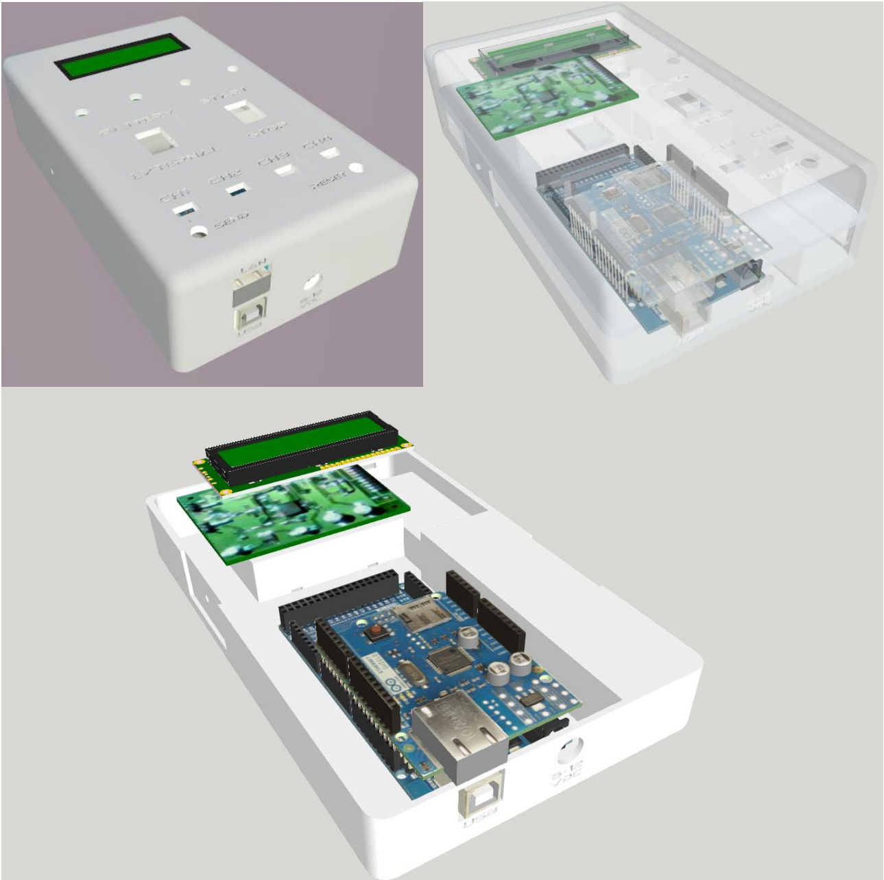
Figure 8 - Case with components without top part
