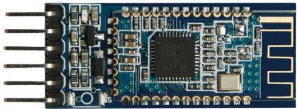
Picture 7: MLT-BT05 Bluetooth module
