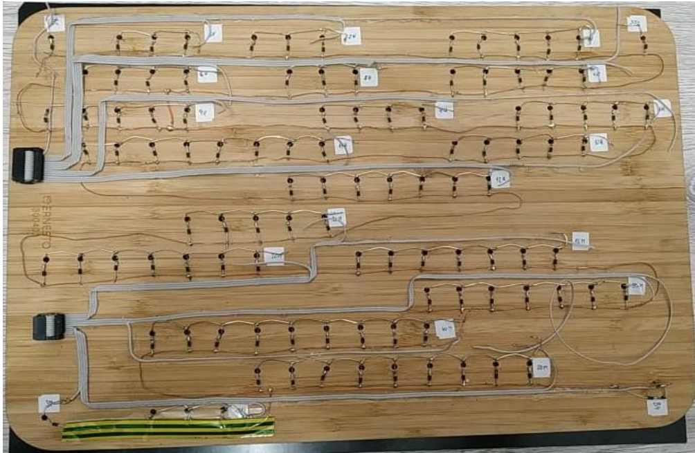
Slovak board with divided IDE cable and connected to LED stripes
