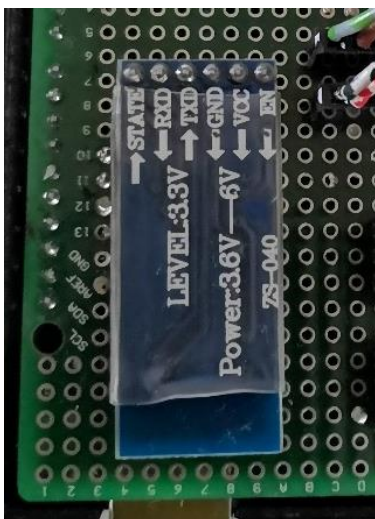
Picture 15: Bluetooth module on the shield
