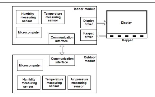
The external unit, situated outside the building, measures climatic data using sensors with the help of microcomputer. The data is transmitted through an interface to the internal unit, situated inside the building. The internal unit processes and displays the received data together with the climatic data, measured by itself. The display mode can be modofied by the help of pushbuttons. We suggest two solutions to the communication through the interface:
